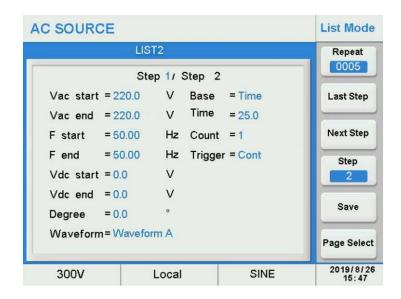
Vac start, F start, Vdc start Waveform parameter in beginning.
